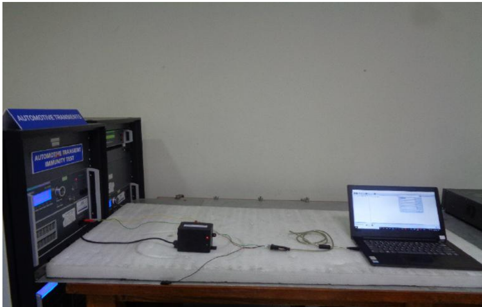
Figure 3: Photograph of Automotive Transient Immunity test setup
