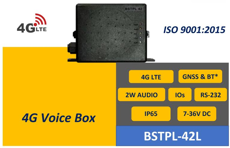
BSTPL-42L VB is an advanced version of voice box used in various applications like automotive, industrial, automation and public places for automated and server-based voice announcements. The Voice Box has provision for broadcasting specific pre-recorded audio messages and support 2-Way voice calling using 4G/LTE and 2G GSM Networks.
